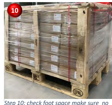
Step 10: check foot space make sure no plastic film or strap on pallet foot!
