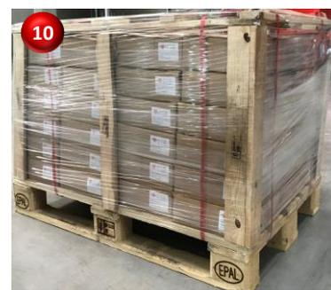
Step 10: check foot space make sure no plastic film or strap on pallet foot!
