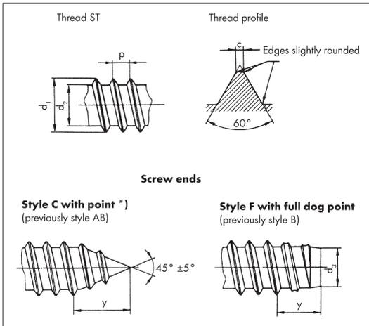
The dimensions for tapping screws such as pitch and diameter are shown in table 48 for ST 1.5 to ST 9.5.
