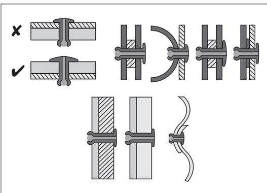
Soft claw blind rivets, blind rivets with a grooved rivet shaft, all-purpose rivets (press clip rivets) are recommended for this application.
