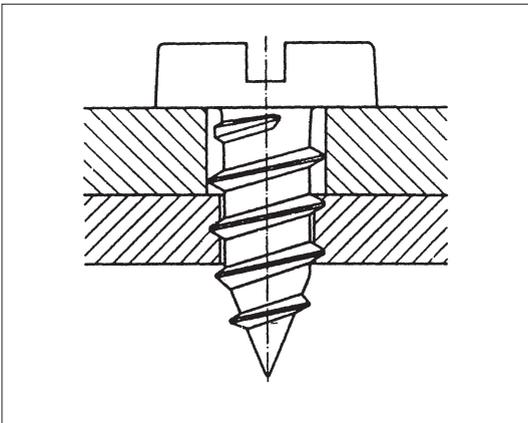
Fig. 2: Simple screwed joint with through hole
