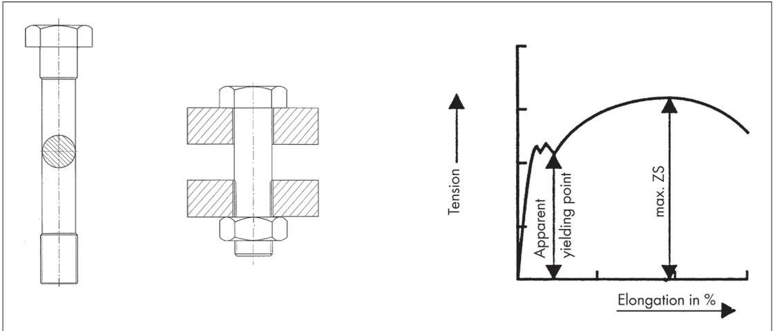
Tensile test on a turned-off screw
