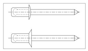
Blind rivet, closed (cup-type blind rivet)
