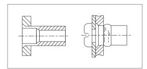
Blind rivet nut, countersunk head
