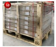
Step 10: check foot space make sure <u>no</u> plastic film or strap on pallet foot!
